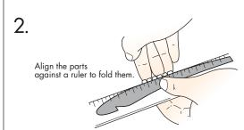
If any of the cut out parts are bent, this will seriously affect the glider's performance. Therefore, be sure to keep all parts perfectly flat till you join them up. For the wings, stabilizer and other parts, use a ruler to give you a proper straight edge to make your folds.
