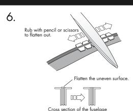
To glue the wings flush onto the fuselage, use a pencil or scissors to flatten out the part where the wings attach to the fuselage.
