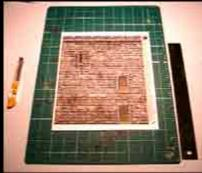
2. Take your metal ruler and place the edge along any of the black guides. IMPORTANT: Apply a strong downward pressure on the ruler. This will keep the template from moving around during cutting.
