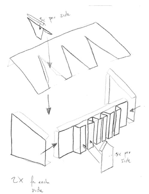
The only tricky thing is the part with the multiple bends. With the illustration it should be no problem as long as you cut and bend correctly as indicated in the PDF file.
