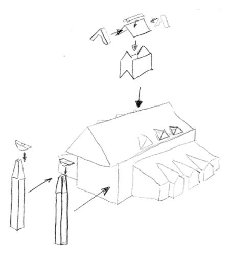
Carefully cut off the overlapping roof in the front where the columns will be fitted. When you try to put the columns into place you will see what I mean.
