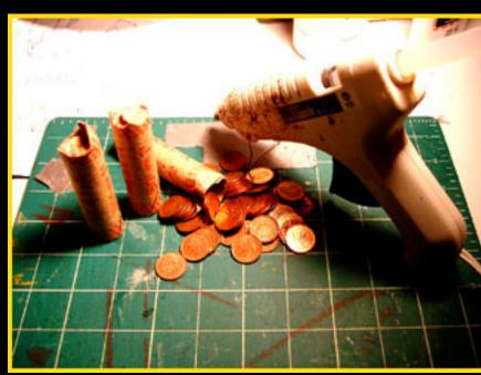
• Penny Stripping is a very simple, speedy process for giving your models some much needed extra weight. This works on small prop pieces right up to large risers. Simply apply pennies to the inside of the model you wish to give weight. The more pennies you add the heavier the model will be. Attach the pennies by using either a strip of tape or a hot glue gun. Because I use my models so often I opted for the glue gun and the pennies have stayed on for months.
