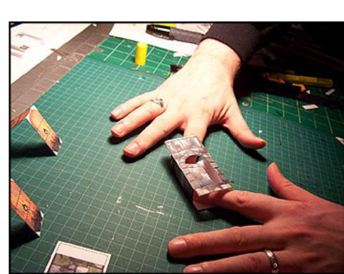
Bend the inner wall tab back and apply a thin bead of glue.
