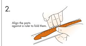
If any of the cut out parts are bent, this will seriously affect the glider's performance. Therefore, be sure to keep all parts perfectly flat till you join them up. For the wings, stabilizer and other parts, use a ruler to give you a proper straight edge to make your folds.
