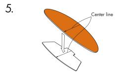
When sticking the right and left wings together, make sure that the center line is not off center.
