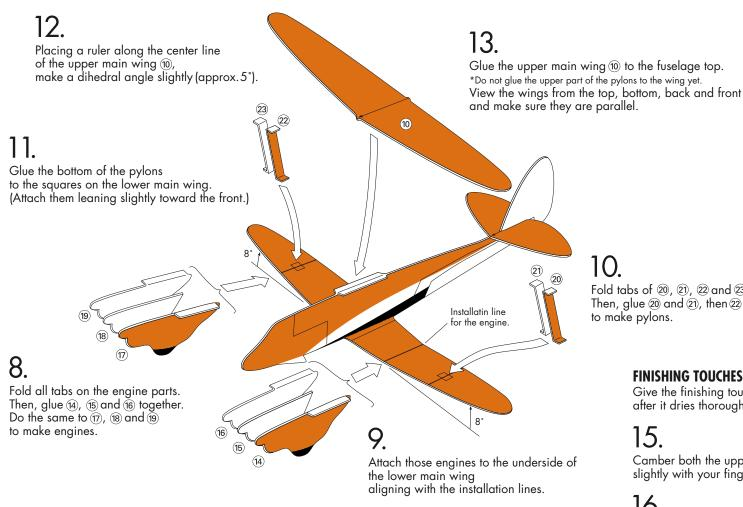
View the plane from the front to check that the fuselage and pylons are parallel. Then, glue the top part of the pylons to the underside of the upper main wing.
