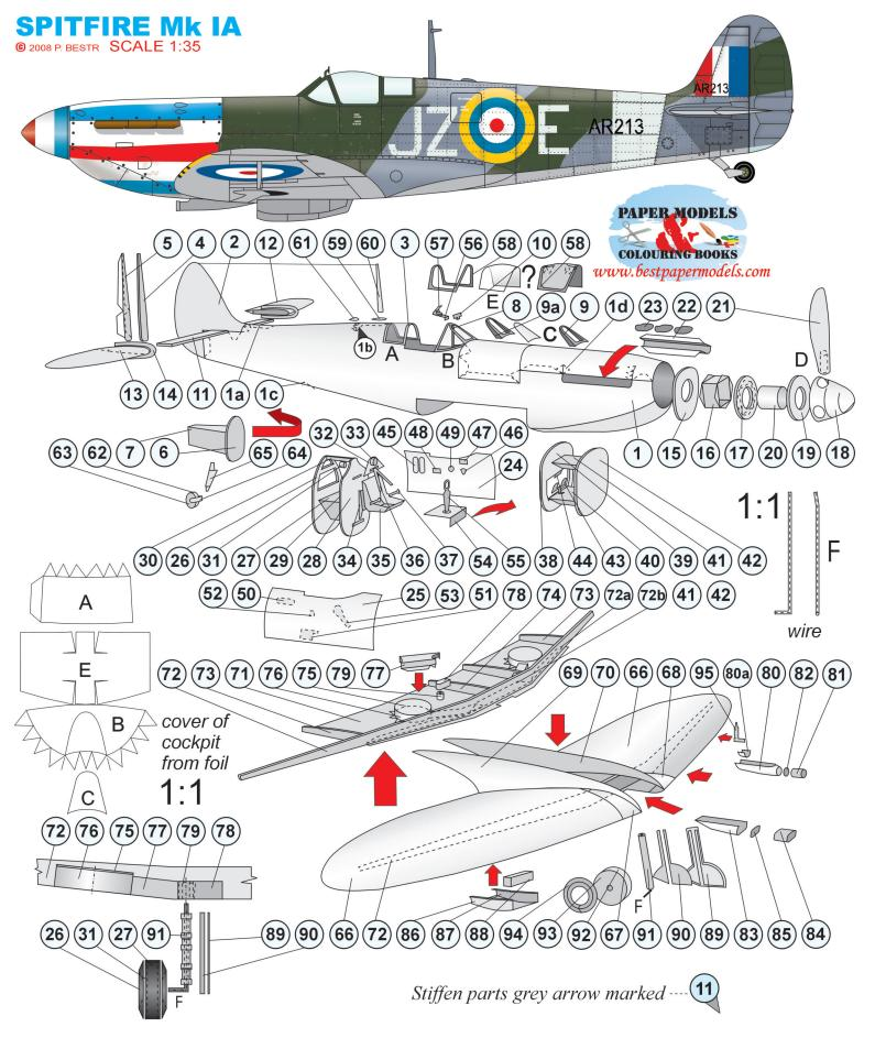
At first prepare fuselage 1 with 1a-1d. Follow with tail 2 and parts 3-14. Then glue engine, propeller 15-21 and exhausts 22, 23. In this time glue cockpit and cover of cockpit 24-58, 58a. Building of fuselage close parts 59-61 and tail gear 62-65. You prepare wing 66-70. Into wing glue parts 71-79 and then wing close. Follow thre coolers 80, 80a, 81-88, covers 89, 90 and main gear 91-94. At least glue part 95.
