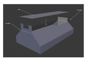
Glue TOP in position and finally glue the MCRN name plague and ship name to the front to complete the stand.
