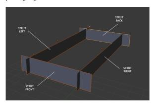
Form the following support structure using the STRUT LEFT, STRUT RIGHT, STRUT FRONT and STRUT BACK.
