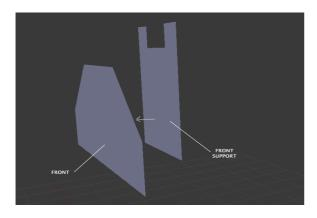
Cut out and glue FRONT SUPPORT to FRONT. Repeat this step for BACK and BACK SUPPORT. Ensure the bottom of both parts line up prior to gluing.
