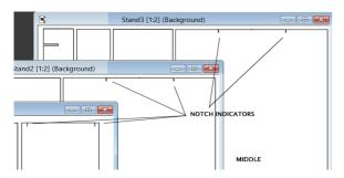
The TOP, MIDDLE and BOTTOM pieces have notch indicators on them. These are in position to show where to cut alignment slots that will help accommodate the FRONT SUPPORT and REAR SUPPORT. Their is no depth indicator as it will depend on the card stock being used to build the stand however 1mm depth is a good start.
