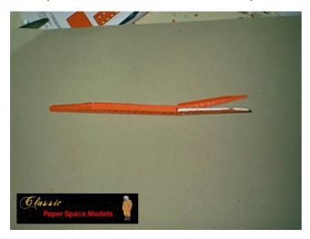
Fold and glue the gantry arm together. It's a good idea to glue 1 flap at a time, and then let it dry a little before continuing. Evt. Shift between the two.
