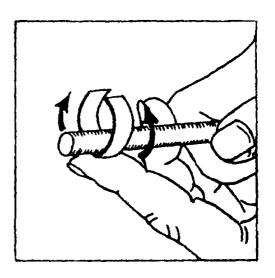
To form a cone use the same procedure as forming a cylinder, but keeping the point of the cone in the same position while forming the curve, i.e. a series of radiating bends.
