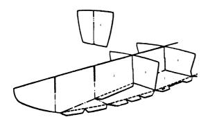
You may wish to use scrap for doubling it to increase the strength. They will fit perfectly and the finished model will be strong enough if used straight from the sheet. However, the structure can be made even stronger by laminating with offcuts of soar sheet or alternatively made from 10 or 20 thou plastic card.
