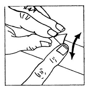
Small strips can be rounded by pulling them between a dull knife blade and the thumb, as one curls a ribbon.
