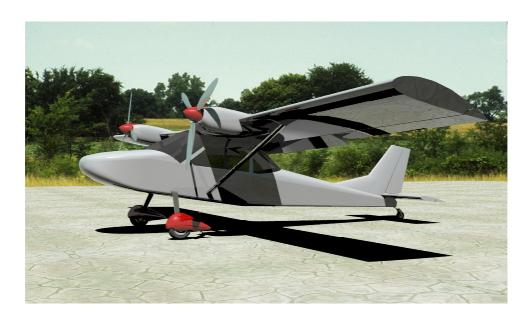
The wing is rectangular with one spar construction supported by spurt over 50% from spread of half wing. The location of rudders is standard. The flaps deflect at three positions 0°, 15° and 30°. The control of ailerons and elevator is with push-pull cables. For the operation of rudder are used classic steel cables. The controlled trim over the elevator is controlled by electric system.
