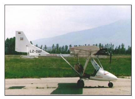
Aluminum alloys 1050, 2024 and 3105 are used as basic building materials. The welded metal parts are made of low carbonic structure steel St20, while turnery and milling parts are of structure steel St45.
