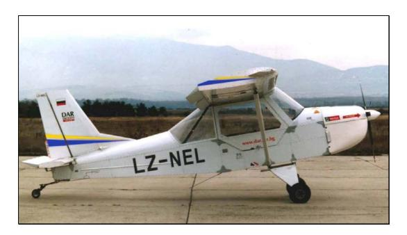
The cabin is fully closed with tandem seats. There is a big door on the right side giving access to seats and cargo sector. The cabin is equipped with all necessary navigation and engine control instruments set in one panel in front of the first seat. The control system is double and allows flying both from front and rear pilot seats.
