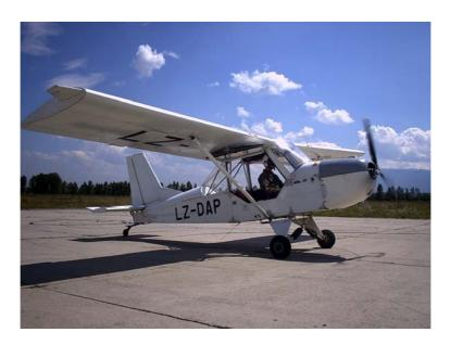
DAR-21 is the first all-metal airplane constructed in Bulgaria. This is the first CAA procedure considering an airplane designed and constructed in Bulgaria as well. All airplanes produced in Bulgaria were constructed by the military forces and never used in civil aviation.
