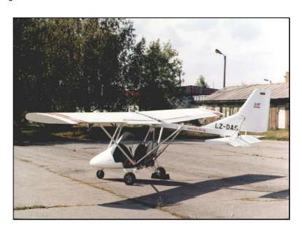
The wing is rectangular with one spar construction supported by spurt over 50% from spread of half wing. The location of rudders is standard. The flaps deflect at three positions 0°, 20°, 40° and 60°. The control of ailerons and elevator is with push-pull cables. For the operation of rudder are used classic steel cables. The controlled trim over the elevator is controlled by electric system.
