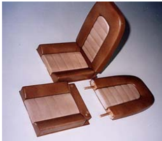
37. Balsa or vacuum formed seats are completed before installation. Attach to landing gear support with wood screws for easy removal.
