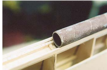
12. Concave wing trailing edge is shaped with sanding tube to match rounded ailerons and flaps.
