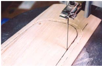
27. Window opening is cut with a scroll saw after routing the edge with a Dremel router.
