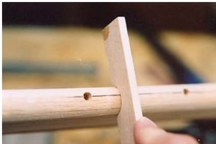
13. Ailerons and flaps leading edges are rounded. Use template for uniform shape. Holes for Robart hinges were drilled before rounding.
