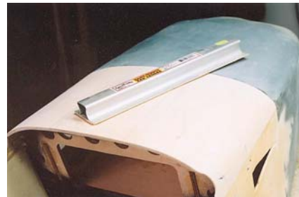
8. Sanding fuselage flush with f/g cowl using a long Great Planes sanding block.
