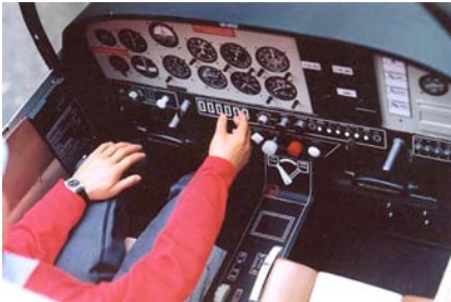
43. Cockpit interior made from common materials. Free graphics are downloadable.
