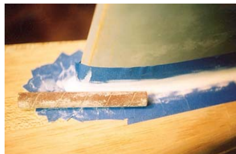
32. Stab fillet is smoothed down to masking tape with a sanding spindle tube before removing masking tape.
