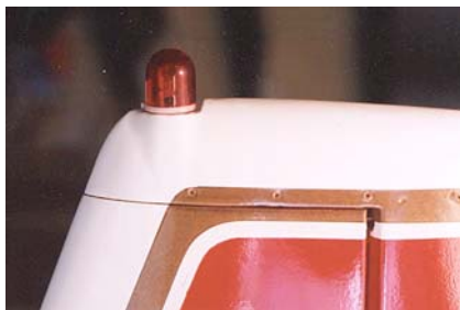
39. Nav beacon light on top of fin is red plastic. Color with RIT dye. RAM LED inside.
