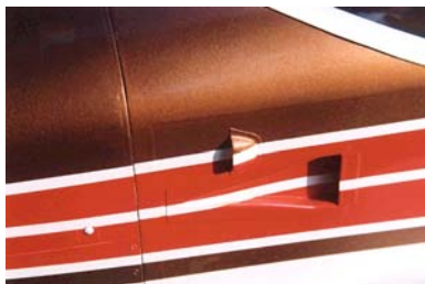
47. Cabin intake and NACA air scoops. Vacuum formed parts available from Aerotech.
