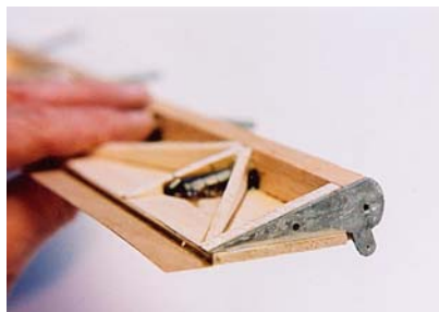
15. Aluminum flap horn is epoxied to end rib. Note ply training edge.
