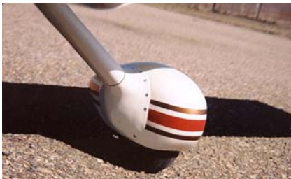
35. Completed main gear. Scale flat head screws in speed fairing match photos of full-sized Lynx.
