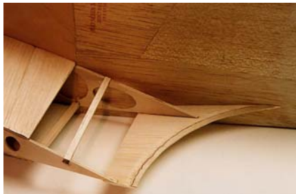
29. Rear wing fillet is installed after joining front and rear fuselage halves. Tapered ply trailing edge.
