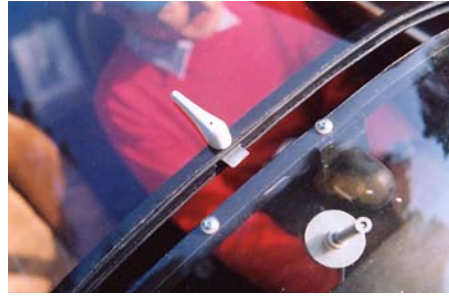
42. Scale canopy latch is a functional alignment key. Canopy and wind-screen are attached to frames with scale screws. Gaskets are black wire insulation CA'ed in place. Temperature probe at lower right.
