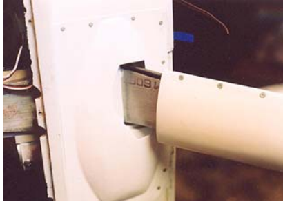
50. Upper speed fairing on main gear leg. Vacuum formed part available from Aerotech. Real rivets and screws are from Micro Fasteners.
