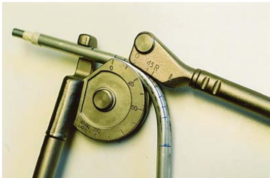
3. Tubing bender tool forms the nose gear strut. Strut can also be purchased.
