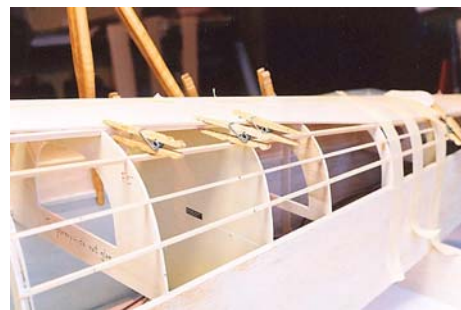
24. Clamp sheeting with masking tape, T-pins and reversed clothes pins while glue sets.
