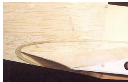
30. \frac{1}{64} " ply forms sheet-metal-like edge of wing fillet.
