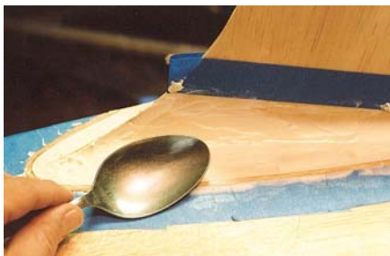
31. Epoxy and SIG microballoons mixture is applied to masked wing fillet with a wet soup spoon.
