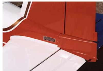
48. Fin is installed after painting. Scale removable tailcone covers rudder servo. Attached with scale screws.
