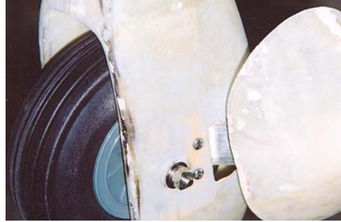
34. Outside of main pant shows threaded axle and two sheet metal screws. Speed fairing is being lowered in place to cover this stuff.
