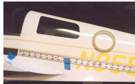
36. Pin stripe 3M Fineline tape is applied over N-number paint masks before spraying red. Straight-edge held in place with masking tape assures straight lines.
