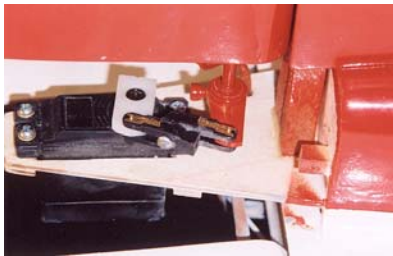
45. Rudder servo with tailcone cover removed. Rudder horn is cut-down nose gear steering arm.
