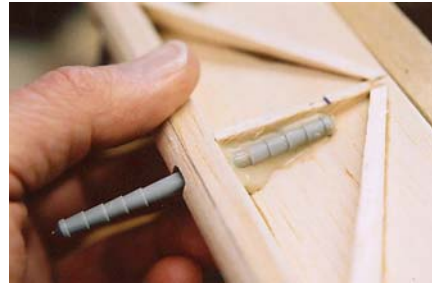
14. Robart aileron and flap hinges are glued in place before top sheeting is added.
