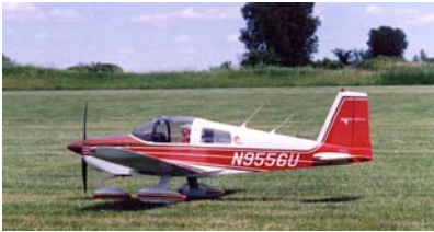
53. In take-off position at a grass field in Minnesota. Sturdy wheel pants work great on grass. 24-inch flying prop is same diameter as scale static prop.
