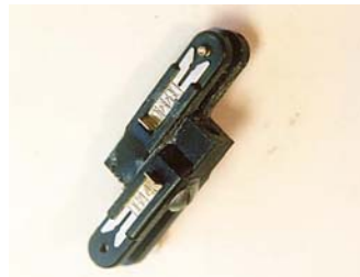
44. World's shortest rudder pushrod—two DUBRO clevises screwed and glued together.
