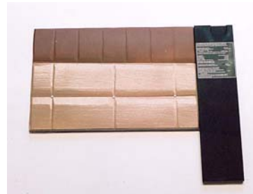
38. Simulated upholstered side panels are assembled and painted before installation. They also cover the canopy screws.
