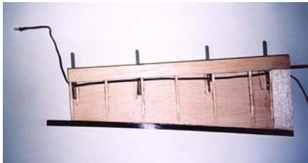
19. Rudder hinges and nav light installed in rudder before sheeting. Carbon fiber strip forms sharp trailing edge.
