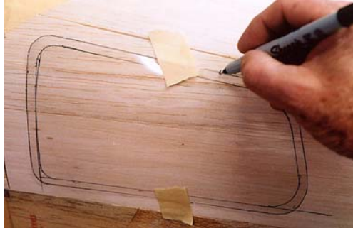
26. Clear plastic window \frac{1}{4} " larger than window opening are traced on fuselage. \frac{1}{4} " thick balsa window frame not glued in place yet.
