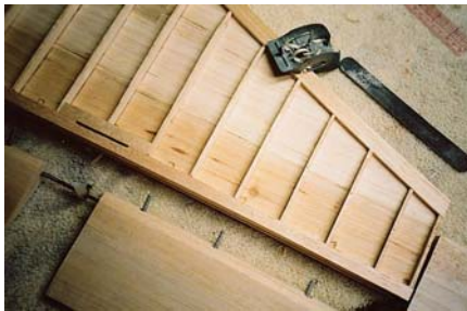
21. Elevator is fitted to stab before stab sheeting is completed. Leading edged tapered with razor plane and sanding stick.
