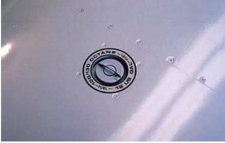
49. Scale gas cap on each wing tip. Graphic available from PRO-MARK. Scale screws are real flat-head screws from Micro Fasteners.
