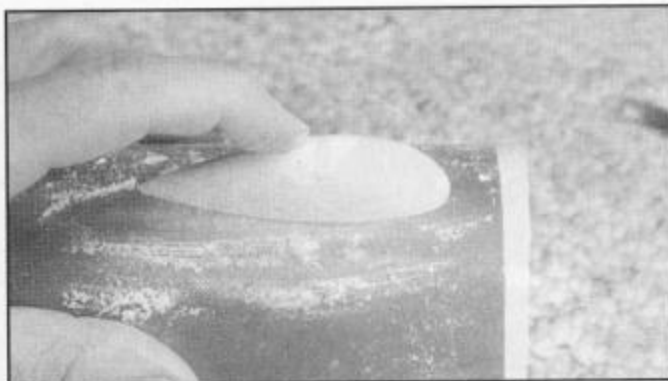
LEFT: Rib stitching is simulated with glue strips and Hair Set Tape. Five rolls required. RIGHT: Fuel cap fairing is fitted to hatch by rubbing on sandpaper, grit side up.
