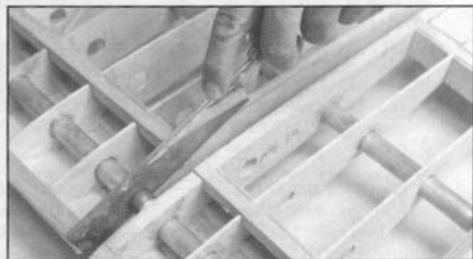
LEFT: Tip is beveled to match outer two ribs. Tested with straightedge before sheeting. RIGHT: Wing tubes are cut after mating wings. Assures perfect alignment.
