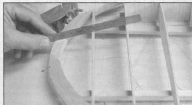
LEFT: Tip is beveled to match outer two ribs. Tested with straightedge before sheeting. RIGHT: Wing tubes are cut after mating wings. Assures perfect alignment.
