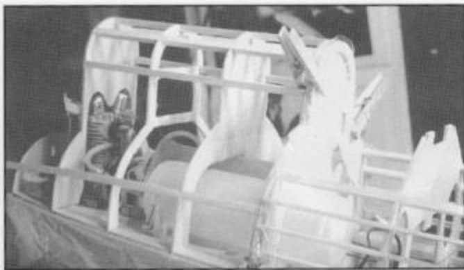
LEFT: After radio and engine installation, cowl frame is assembled in place. Saran Wrap prevents gluing to framework. RIGHT: Rear of fuselage ready to accept tail. Dual-clevis carbon fiber elevator pushrod in place.
