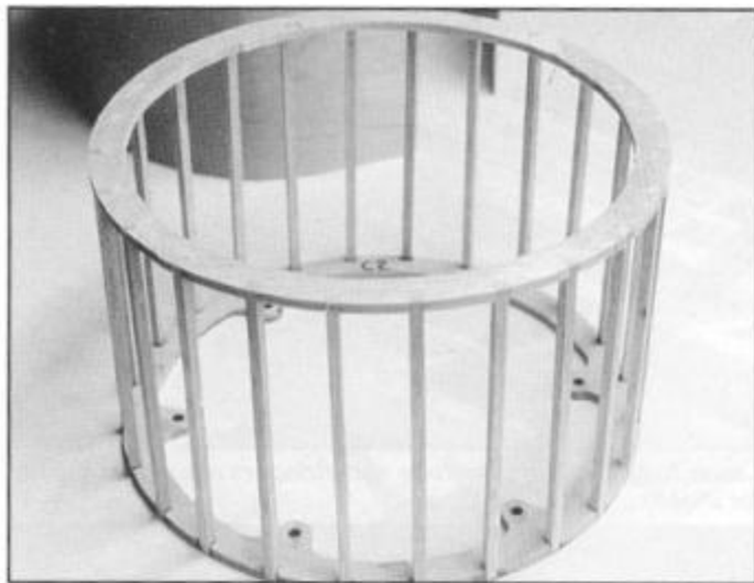
ABOVE: Use the template to shape the balsa nose bowl. LEFT: Wood cowl form ready for 1/32" ply covering.
