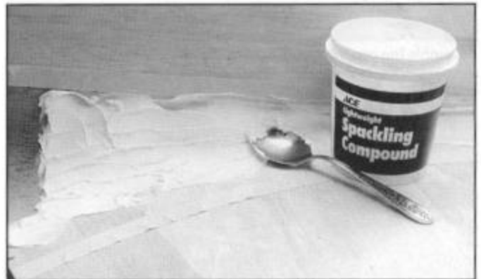
Center wing fillet is formed with spackling and a tablespoon. Double-thick masking tape defines the edge.
