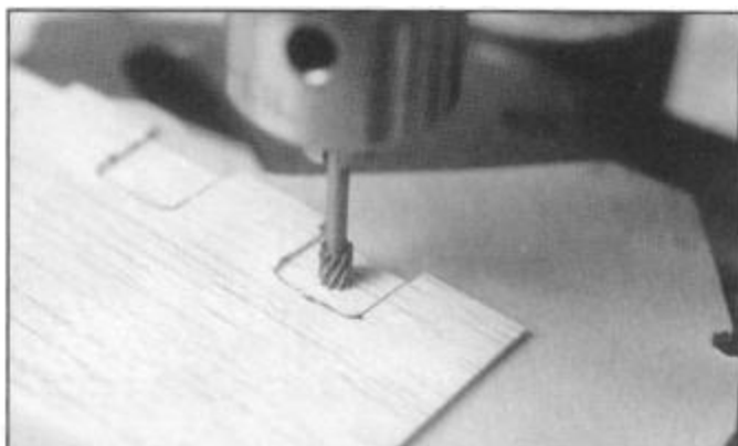
Flap core routed to recess Klett hinges. Dremel straight bit in a drill press.
